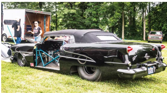
Kerm Shindledecker's Oldsmobile has a hand-built fiberglass body and is powered by a stroked Olds engine.
